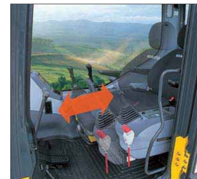
Seat Sliding Amount: 340 mm 13.4", increased 120 mm 4.7"
