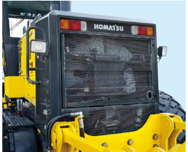
Hydraulic driven cooling fan
