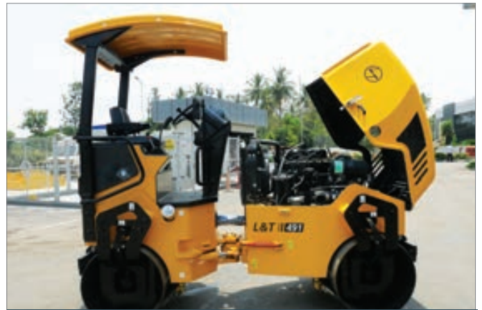
Ground Level Service Access
